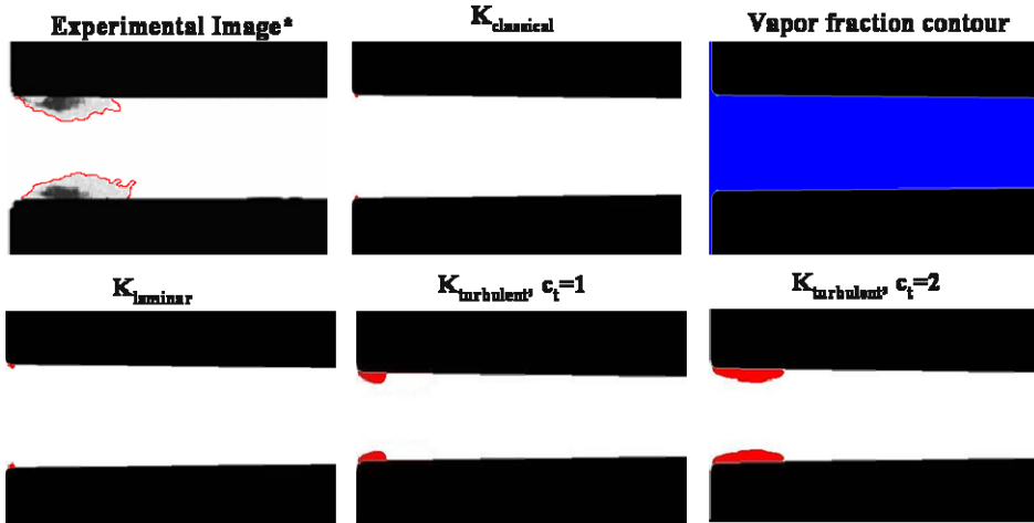
Fig. 1. Comparison between the measured (Winklhofer, 2001), predicted vapor fraction contours, and cavitation inception regions predicted by different cavitation criteria. The injection and back pressures are 100bar and 40bar respectively.
