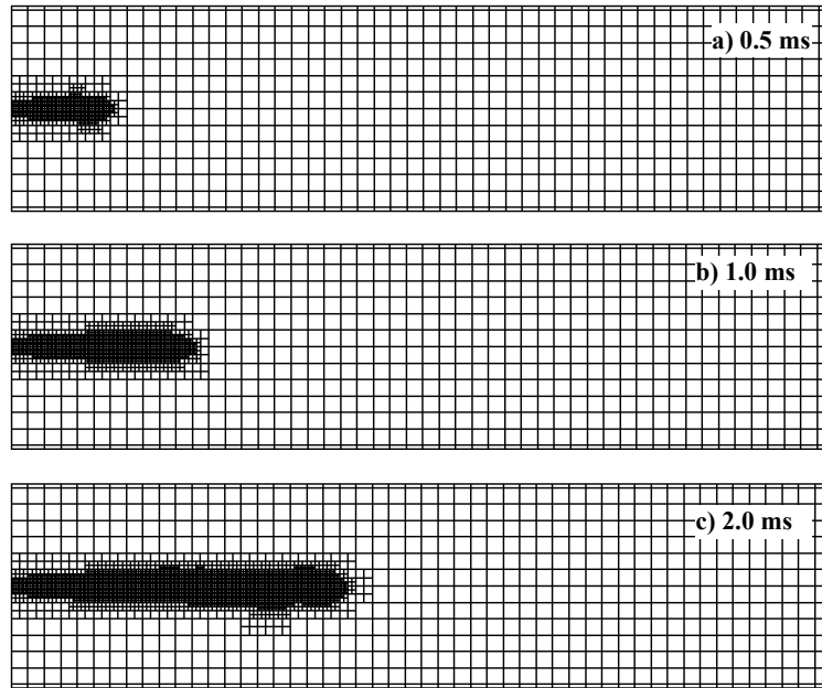
Fig. 2 Grid generated in CONVERGE at different times during the simulation for non-evaporating sprays described in Table 1. The field of view in the axial and radial direction is about 200 and 50 mm, respectively
